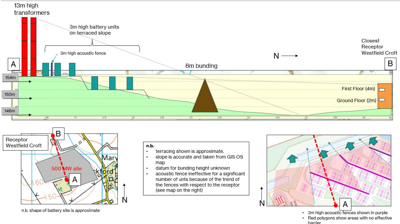
**Appendix 1** provides an illustrative site–receptor cross-section (slope is accurate and extracted from an OS map) using conservative assumptions for plant height, boundary mitigation, and receptor height. While illustrative and not an acoustic model, it demonstrates the type of geometric relationship that the noise assessment itself should have presented and highlights why effective screening—particularly to first-floor receptors—cannot be assumed without explicit evidence.
